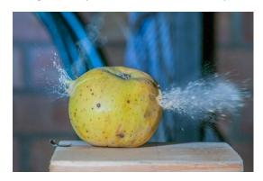
as a balloon bursting. On the theme of destroying things there is a projectile sensor available that allows the Camera Axe to calculate the speed of a projectile, such as an airgun pellet and then by entering the distance to the target will fire the flash at the appropriate time when the pellet hits it. Old Christmas tree baubles and apples come to mind although they do make a mess and best done in the garage!
